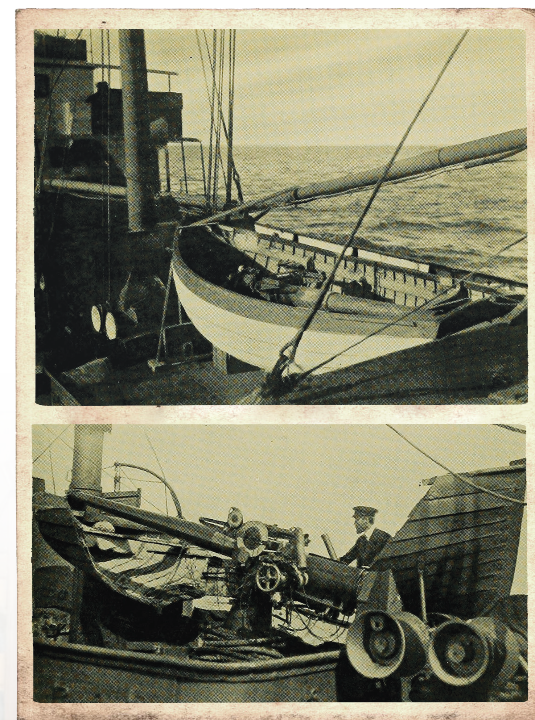
Above: These two photographs show how Penshurst expertly disguised its true purpose. This dummy boat can be quickly pulled aside, allowing the hidden 12-pounder gun to be brought to bear on an enemy target in a matter of seconds. Originally published in the Q-Ships and their Story by E Keble Chatterton, 1922.
