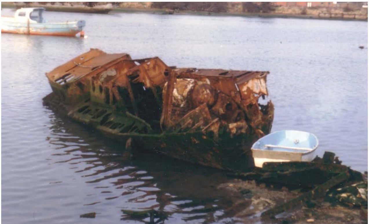
FIGURE 5: PINNACE 704 IN THE 1980s, THOUGHT TO BE 1987, WHEN THE BOW OF THE VESSEL AND GUN MOUNT HAS BEEN TRUNCATED, BUT WHERE LARGE PARTS OF THE MAIN SUPERSTRUCTURE ARE STILL IN PLACE. THE BOILER IS NOW CLEARLY VISIBLE WITHIN THE FORWARD PART OF THE VESSEL (IMAGE: COURTESY OF PHILIP SIMONS).
