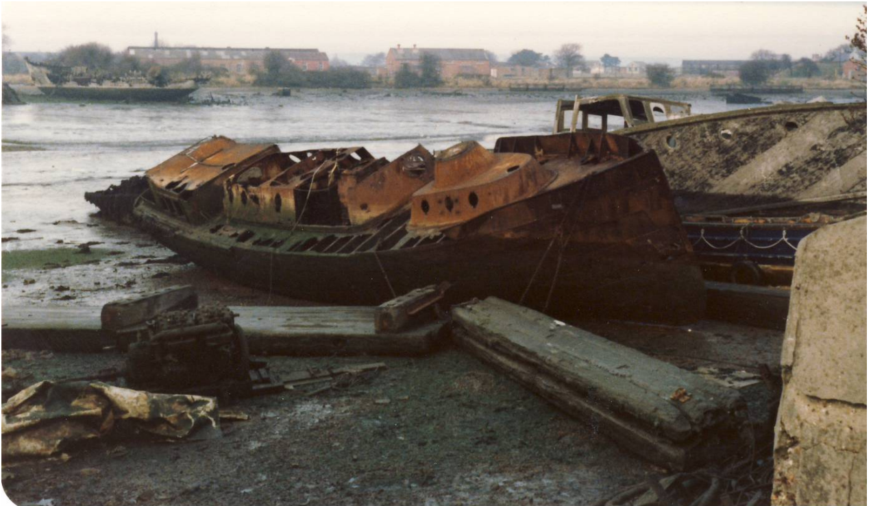
FIGURE 4: PINNACE 704 PHOTOGRAPHED AT AN UNKNOWN DATE. ASSUMED TO BE AFTER FIGURE 3 BECAUSE OF THE ABSENCE OF THE STARBOARD RUBBING STRAKE, AND CLEARLY PRIOR TO THE TRUNCATION OF THE BOW, VISIBLE IN FIGURE 5 (IMAGE: COURTESY OF PHILIP SIMONS).
