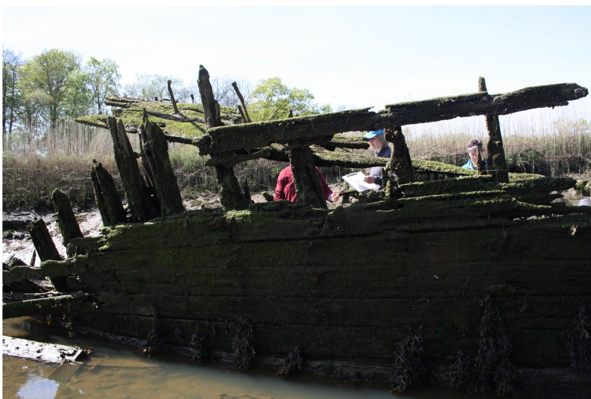
FIGURE 11: OUTER VIEW OF THE STARBOARD SIDE OF THE WESSEX IN 2016, DEMONSTRATING THE LOSS TO THE INNER AND OUTER PLANKING AND THE FRAMES.
